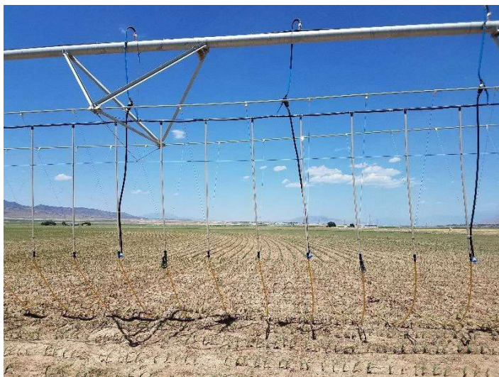
Figure 3. The filters can be seen on the feed lines from the pivot pipe above. Whole system filtration near the pump is recommended if the entire pivot uses MDI. The ties used to keep the rigid drops vertical can also be seen secured to the truss rods. Photo by Troy Peters.
