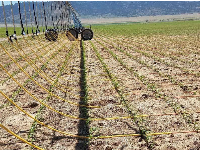
Figure 2. An MDI system that uses rigid drops. Photo by Troy Peters.
