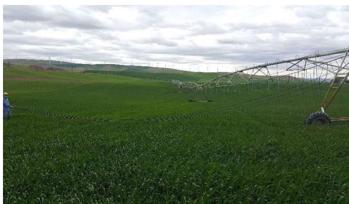
Figure 4. MDI installed on a center pivot while retaining the sprinklers for switching between MDI and MESA. The driplines on the outside spans of the pivot are longer since it covers a larger area in the field. Although the crop is wheat, the MDI system is set up for taller crops. Photo by Behnaz Molaei.
